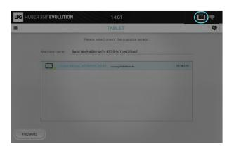
Your device automatically detects your tablet. The "**tablet**" icon at the top right corner of your device screen and that of your tablet ensures that the connection is operational.
