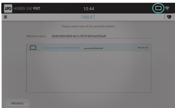
Your device automatically detects your tablet. The “**tablet**” icon at the top right corner of your device screen and that of your tablet ensures that the connection is operational.
